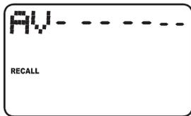
Remarks: (1) if lap counter is > 99 or either Lap or split is greater than 9 hours 59 min 59.99 sec, the power of the computer has been exceeded and AV information will be disabled as shown. (2) if either lap of split is greater than 9 hours 59 min 59.99 sec, the power of the computer has been exceeded and the SL and FS information will be disabled.
