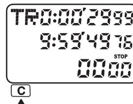
Remarks: (1) if the preset time is 29 seconds, only 2 beeps will sound on approach of zero. (2) When timer reaches zero while the stopwatch is in other modes, only 2 beeps will sound.
